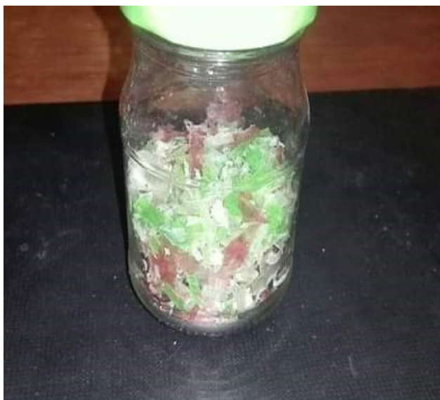
Figure 18. Shreds or pallets of hard bioplastic that can be used in moulding process for the creation of hard type kitchenware like spoons and plates.
