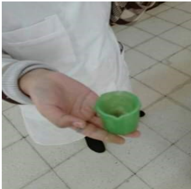
Figure 14. Example of moulding a mass of bio-plastic into a beaker shape, see also Results & Discussion section chapter.
