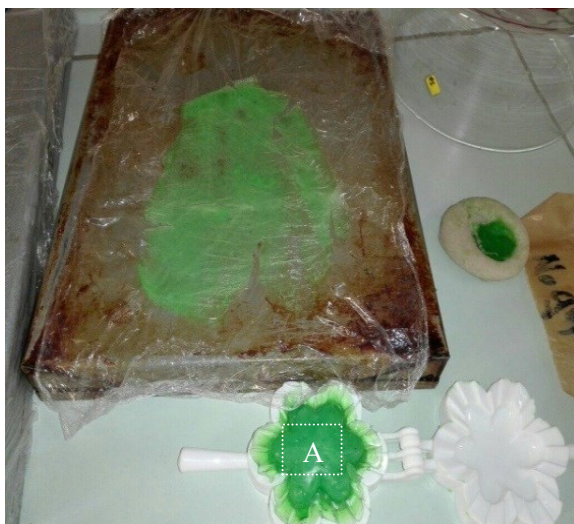
Figure 19. Flexible bioplastic coloured green; in thick and flower shaped blob using a press mould.
