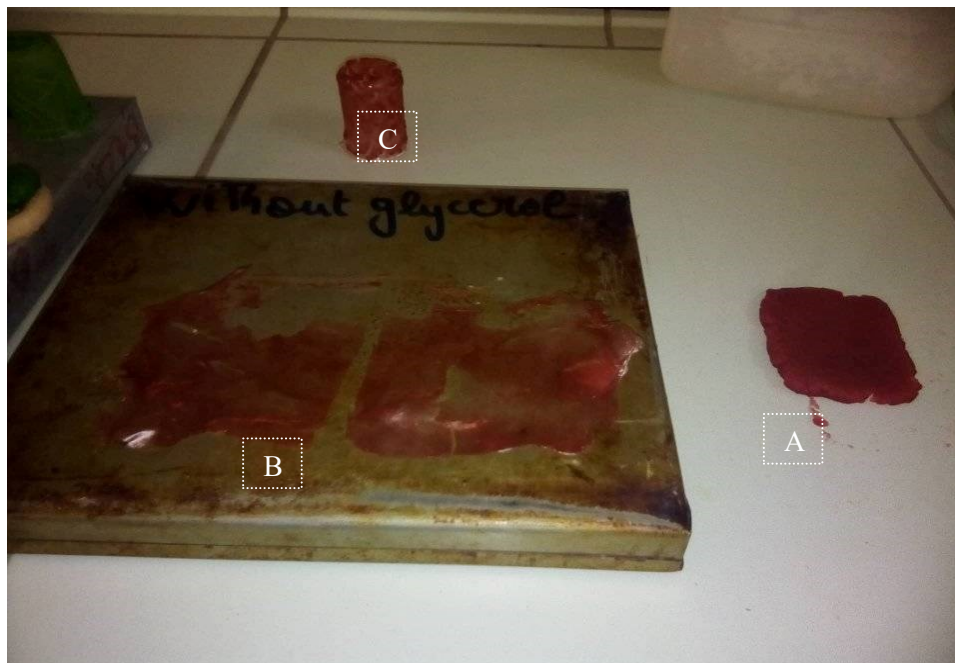
Figure 17. Hard bioplastic coloured red; A 1cm thick block, B crackable sheet and C beaker shaped mould.
