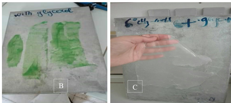
Figure 20. Transparent flexible bioplastic film can target packaging, storing food industry and may be used as alternative to plastic bags.
