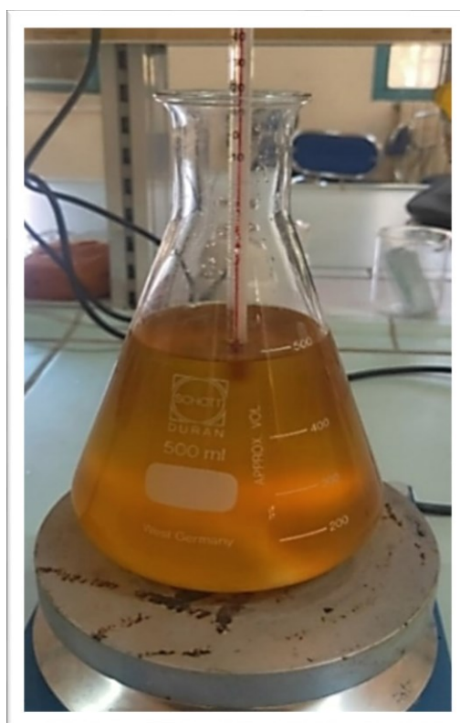
Figure2. Mixture of Sodium methoxide solution with used cooking oil.
